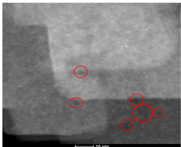
Fig. 15 High-resolution HAADF-STEM image of 1 wt% Pd/SSZ13 with Si/Al ratio 6 after hydrothermal aging at 750 °C for 16 h in 10% H 2 O/air flow. The bright spots are Pd entities in the pores
